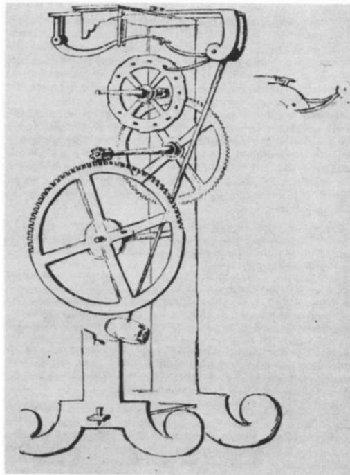
**Fig. 5.** Pendulum clock conceived by Galileo Galilei around 1637. The earliest known pendulum clock design, it was never completed.
