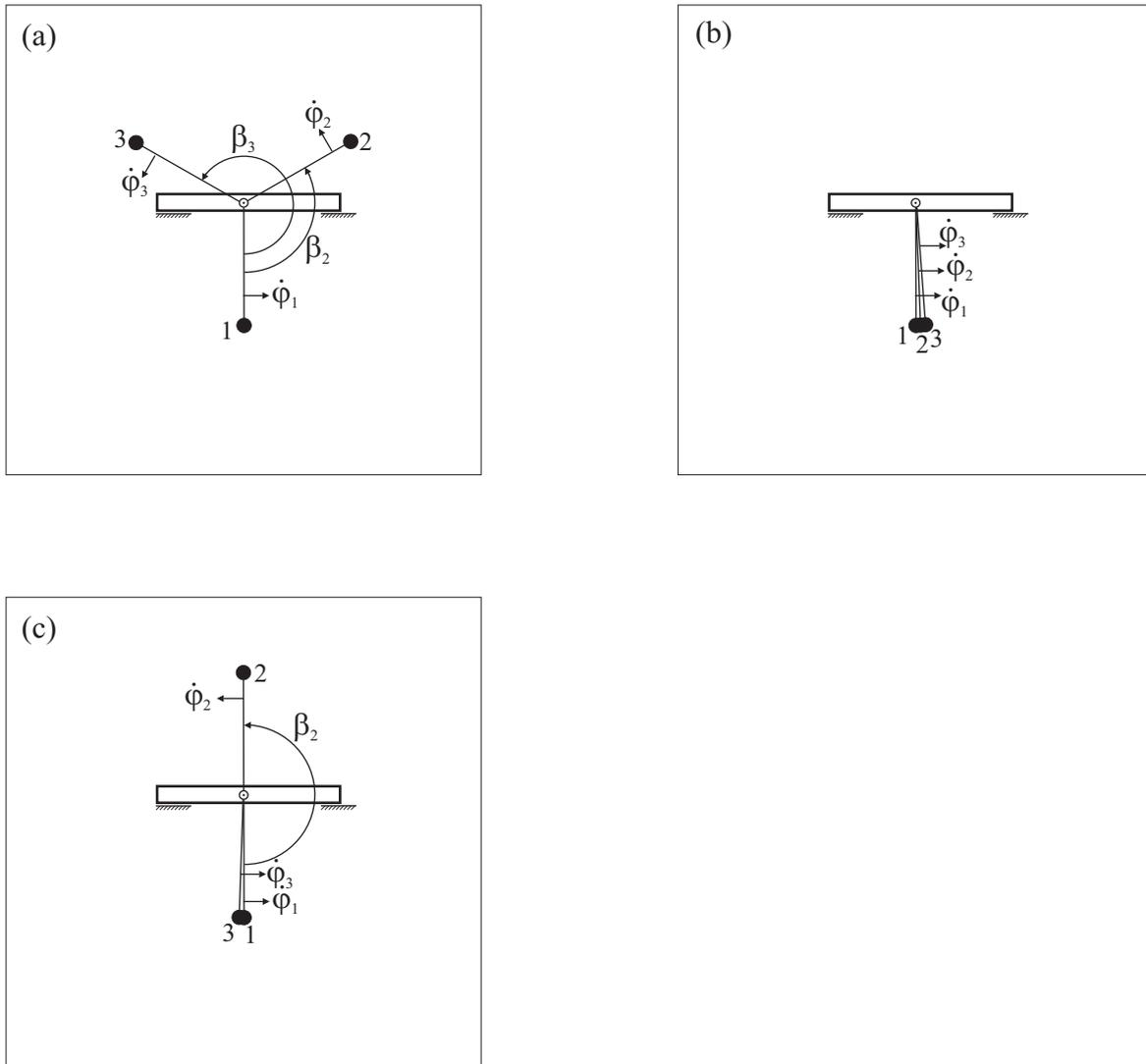
Fig. 7: Synchronization configurations in the system (1-2) with  $n=3$  pendulums; (a) phase synchronization with phase shifts between pendulums:  $\beta_1=0.0^\circ$ ,  $\beta_2=120.0^\circ$  i  $\beta_3=240.0^\circ$ , (b) complete synchronization ( $\beta_1 = \beta_2 = \beta_3=0$ ), (c) antiphase synchronization of a single pendulum with the cluster of two other pendulums,  $\beta_1=0.0^\circ$ ,  $\beta_2=180.0^\circ$  i  $\beta_3=0.0^\circ$ .
