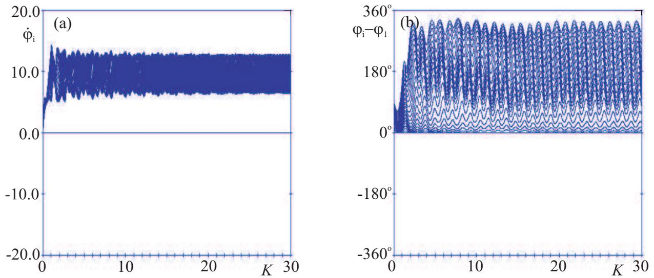
Fig. 9: Phase synchronization of  $n = 20$  pendulums in the system (1-2):  $m_1 = m_2 = \dots = m_{20} = 1.00$ ,  $l = 0.25$ ,  $c_\varphi = 0.01$ ,  $N_0 = 5.00$ ,  $N_1 = 0.50$ ,  $k_x = 1000.0$ ,  $M = 20.0$ ,  $\varphi_{i0} = \frac{i \times 90^\circ}{20}$ ,  $\dot{\varphi}_{i0} = 0.0$ ; (a) pendulums' velocities  $\dot{\varphi}_i$ , (b) angular displacements  $\varphi_i - \varphi_1$ .
