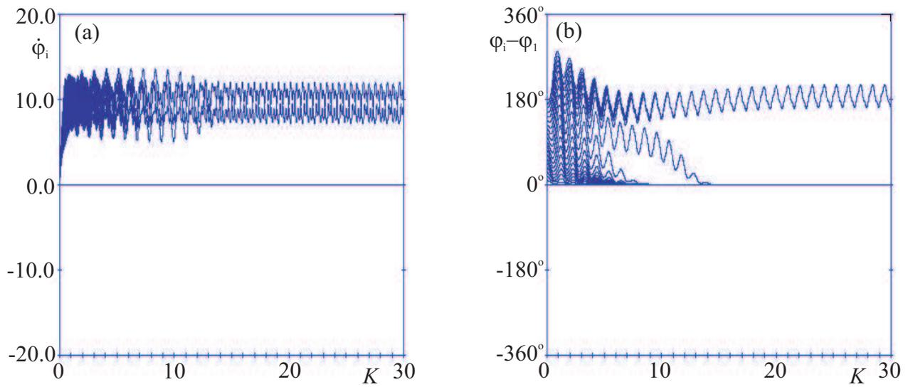
Fig. 11: Cluster synchronization of 20 pendulums in system (1-2):  $m_1 = m_2 = \dots = m_{20} = 1.00$ ,  $l = 0.25$ ,  $c_\varphi = 0.01$ ,  $N_0 = 5.00$ ,  $N_1 = 0.50$ ,  $k_x = 20000.0$ ,  $M = 20.0$ ,  $\varphi_{i0} = \frac{i \times 180^\circ}{20}$ ,  $\dot{\varphi}_{i0} = 0.0$ ; (a) pendulums velocities  $\dot{\varphi}_i$ , (b) angular displacements  $\varphi_i - \varphi_1$ . Clusters of 7 and 13 pendulums are synchronized in antiphase.
