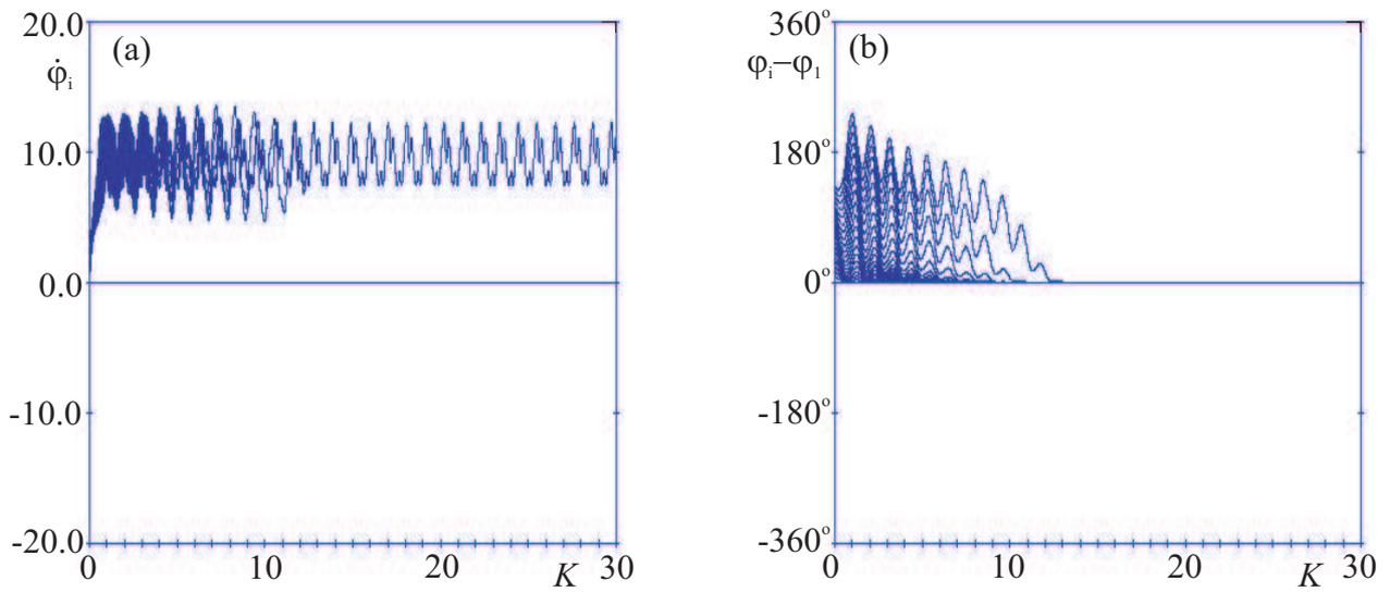
Fig. 10: Complete synchronization of 20 pendulums in system (1-2):  $m_1 = m_2 = \dots = m_{20} = 1.00$ ,  $l = 0.25$ ,  $c_\varphi = 0.01$ ,  $N_0 = 5.00$ ,  $N_1 = 0.50$ ,  $k_x = 20000.0$ ,  $M = 20.0$ ,  $\varphi_{i0} = \frac{i \times 140^\circ}{20}$ ,  $\dot{\varphi}_{i0} = 0.0$ ; (a) pendulums velocities  $\dot{\varphi}_i$ , (b) angular displacements  $\varphi_i - \varphi_1$
