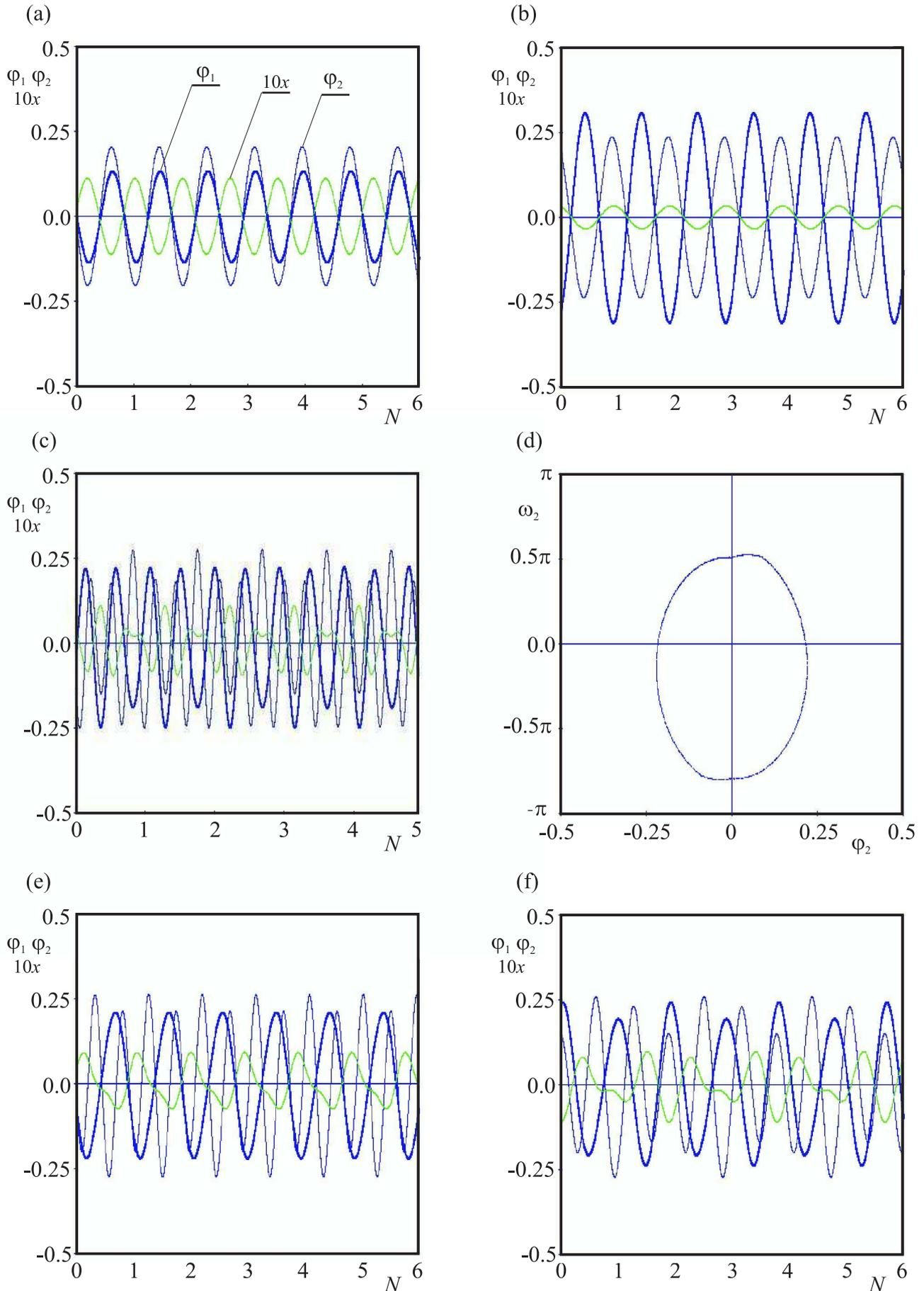
Fig. 7: Different types of synchronization of the clocks pendulums; (a) 1:1 in-phase synchronization for  $\xi = 0.95$ ; (b) 1:1 anti-phase synchronization for  $\xi = 0.95$ ; (c) time series of quasiperiodic motion for  $\xi = 0.6871$ ; (d) Poincare map, (e) synchronization 1:2 for  $\xi = 0.51$ ; (f) synchronization 2:3 for  $\xi = 0.6887$ .
