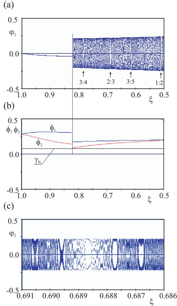
Fig. 6: (a) bifurcation diagram of the system (1) for increasing  $\xi$ ; (b) minima of amplitudes of pendulums' oscillations; (c) enlargement of (a) in the neighborhood of 2:3 synchronization.
