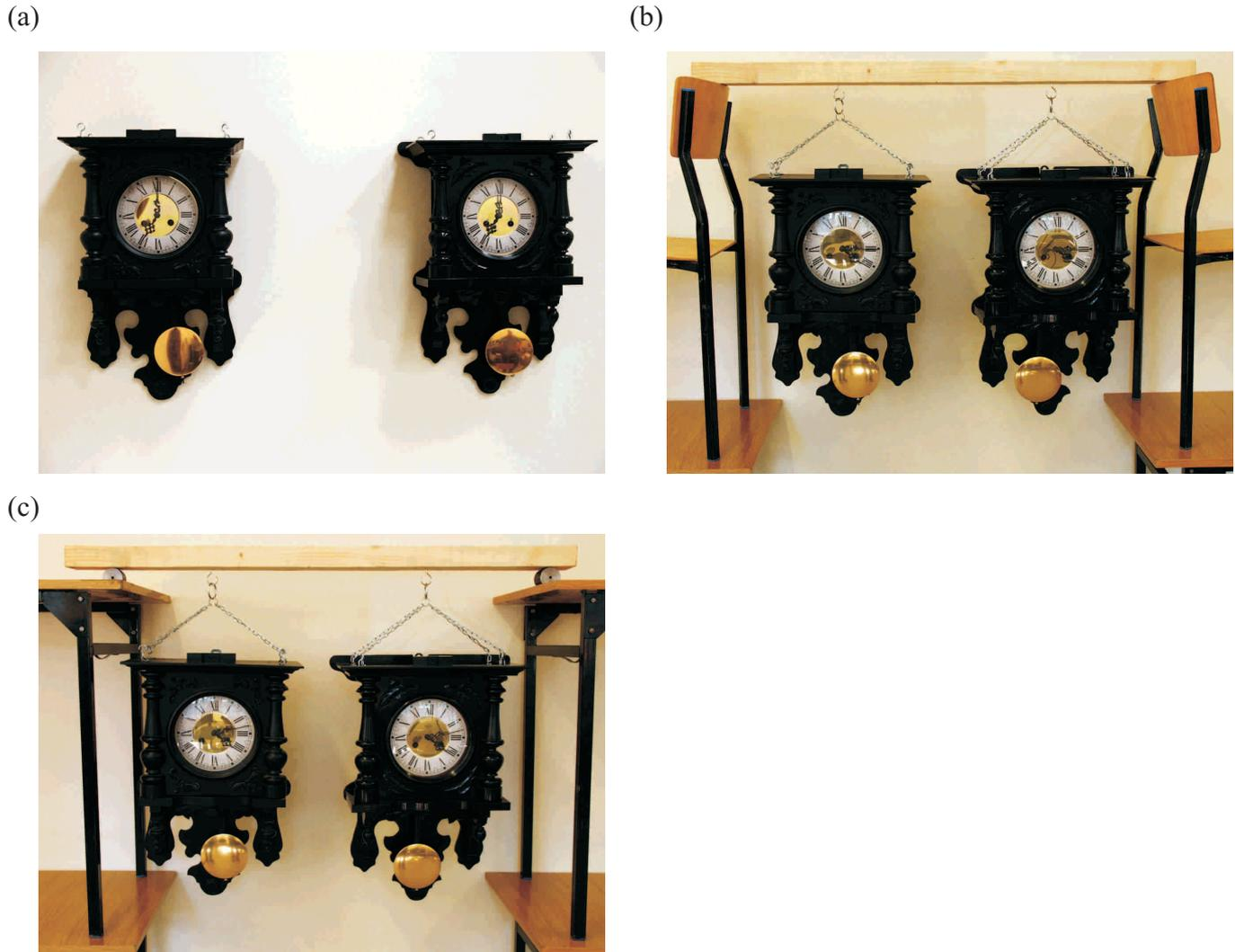
Fig. 2: Experiments with two pendulum clocks: (a) clocks hang on the wall, (b) clocks hang from the beam located on the chairs' backs, (c) clocks hang from the beam which can roll horizontally on the tables' desks.
