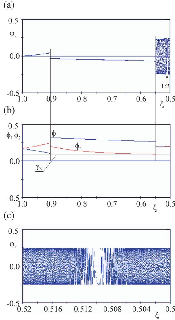
Fig. 5: (a) bifurcation diagram of the system (1) for decreasing  $\xi$ ;  $\varphi_{10} = \varphi_{20} = 0.26$ , end with  $\xi = 0.5$ ; (b) minima of amplitudes of pendulums oscillations; (c) enlargement of (a) in the neighborhood of 1:2 synchronization.
