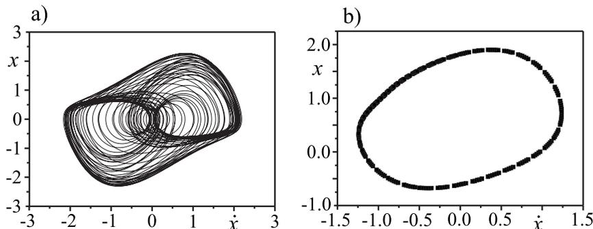
FIG. 1. Quasiperiodic motion of the VDP oscillator: (a) Phase plane and (b) Poincaré section.
