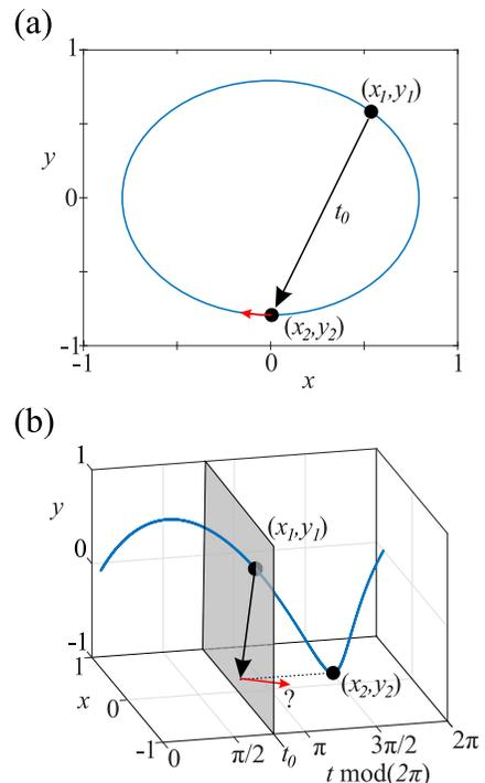
FIG. 2. Presentation of the exemplary periodic attractor of a 2-dimensional autonomous (a) and a non-autonomous (b) system. Both points  $(x_1, y_1)$  and  $(x_2, y_2)$  belong to the attractor. The black arrows indicate the effects of perturbation that occurs at time  $t_0$ .
