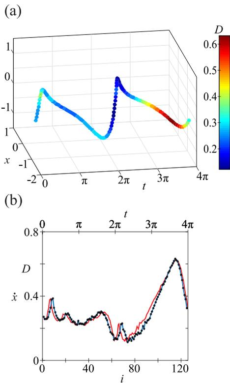
FIG. 5. Attractor  $F$  of the Duffing system (Eq. 6) with middle points of 125 segments marked by dots colored according to the value of  $D$  - panel (a). Evolution of the stability margin  $D$  along attractor  $F$  with respect to the number of segment. With black dots we indicate the value of  $D$  in the middle of segment and with blue line its continuous estimation (b).
