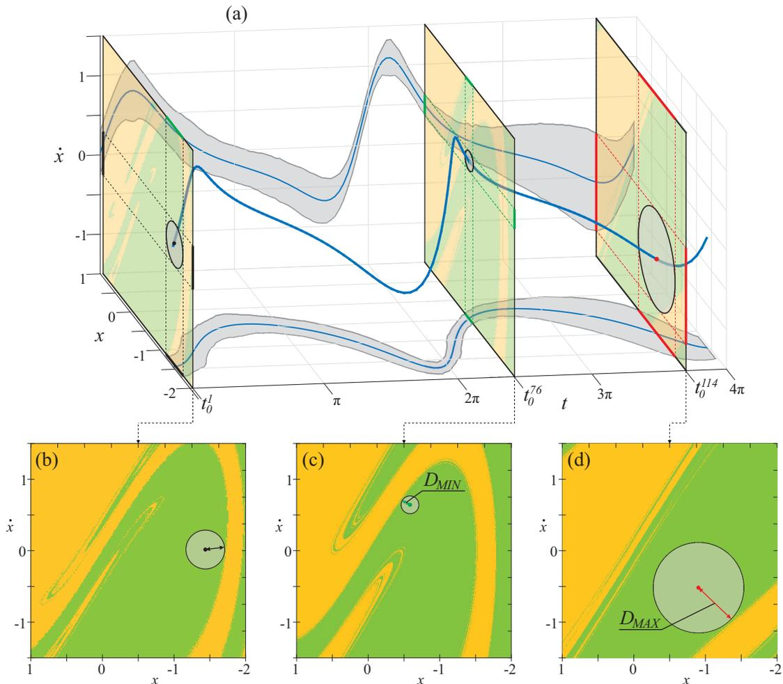
FIG. 6. Panel (a) is a 3D presentation of solution  $F$  with the evolution of measure  $D$  in time domain. Three exemplary basins of attraction calculated for  $t^1$ ,  $t^{76}$  and  $t^{114}$  are shown in panels (b,c,d).
